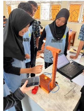
Figure 1. Implementation of the infrared sensor-based pendulum apparatus during guided inquiry learning on SHM.
